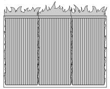
Figure 22 - Incorrect Burner Flame Pattern
